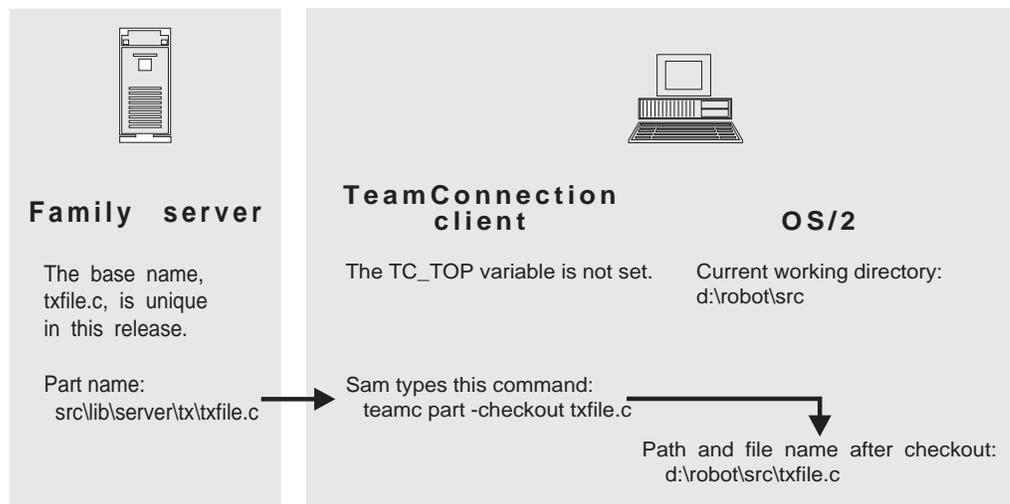
Next Sam needs to check out \src\lib\server\tx\msg.h. Because other files named msg.h exist in release **9501**, he must specify the entire path name.
